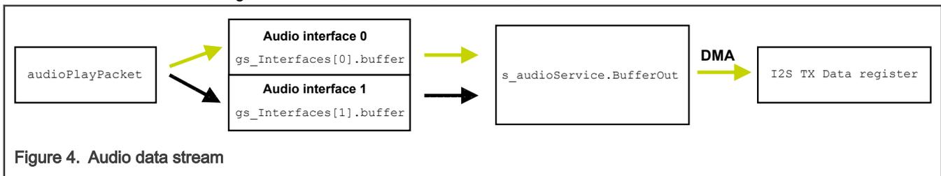
In this example, only one audio interface is implemented and the function of audio mixer is not used, that is, the audio data stream only moves according to the direction of the green arrow of [Figure 4](#).
