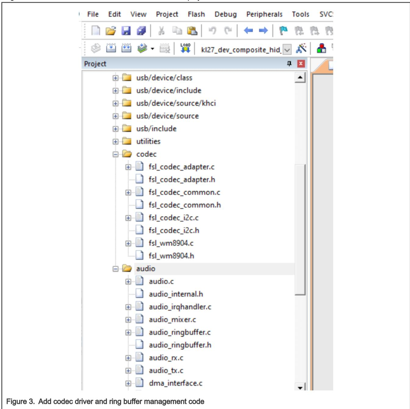
Figure 3. Add codec driver and ring buffer management code
