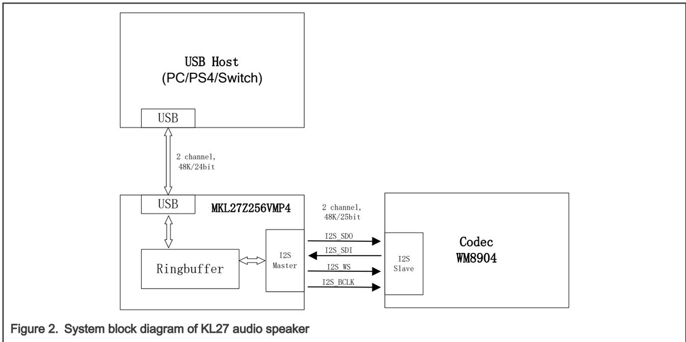
Figure 2. System block diagram of KL27 audio speaker
