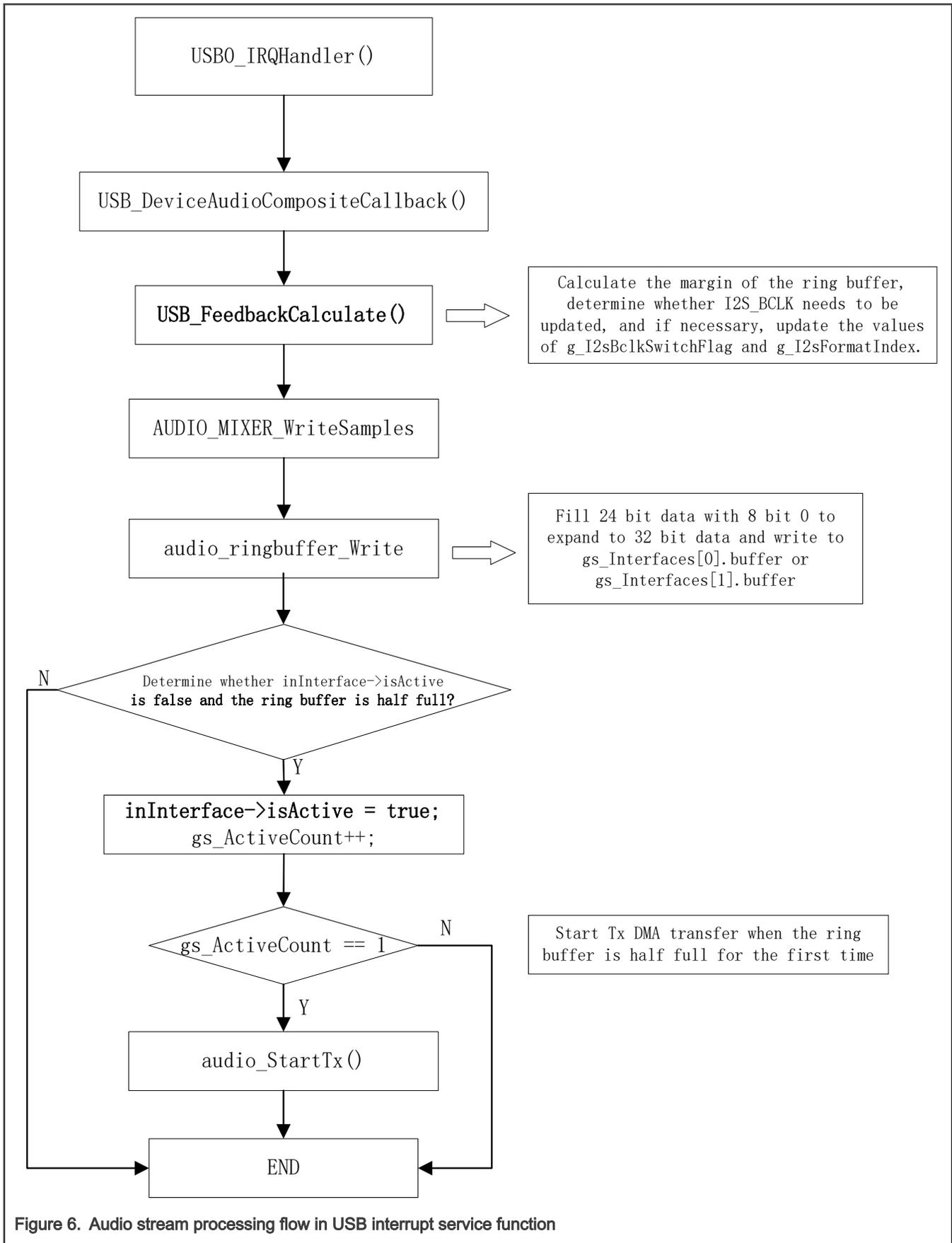
Figure 6. Audio stream processing flow in USB interrupt service function
