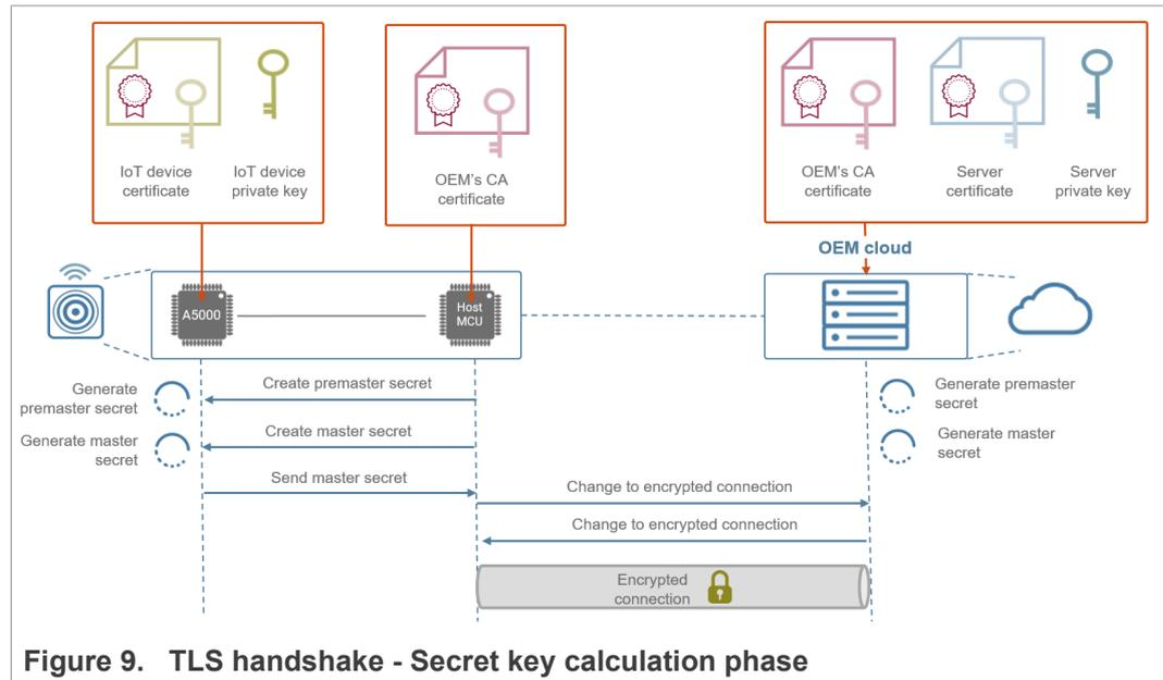
At this point, both the IoT device and the OEM cloud are in possession of the shared secret key and can start to securely exchange data using a symmetric cryptographic algorithm.
