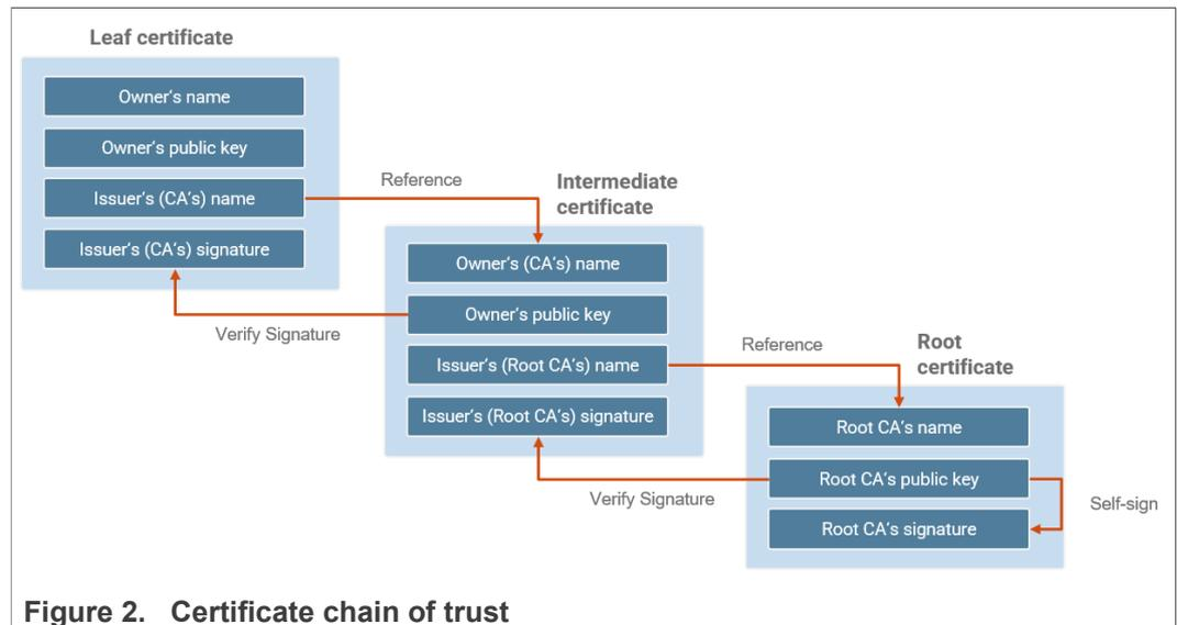
IoT devices manufactured by the OEM should be equipped with a unique key pair and a digital certificate signed by the OEM's CA certificate. The OEM's CA certificate is used to sign all the certificates of the devices manufactured by the OEM as shown in [Figure 3](#). Precisely, this signature provides the means to verify the validity of device certificates in the field.
