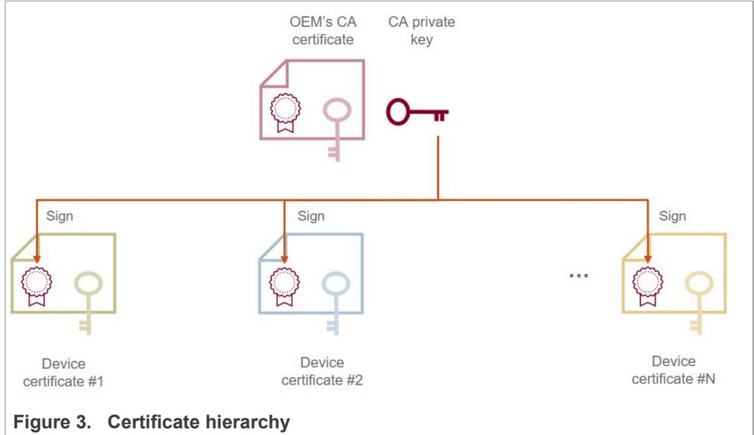
Before an IoT device manufactured by the OEM goes to the operation phase, they must possess the CA certificate, a device certificate and a key pair securely stored. Similarly, the OEM cloud platform must possess a certificated signed by the CA and its related private key as shown in [Figure 4](#).
