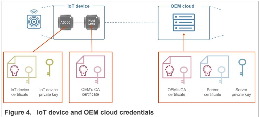
Security ICs chips like A5000 are capable of internally protecting private keys in IoT devices. The CA certificate is typically stored outside the A5000. [Section 4](#) outlines the A5000 trust provisioning models available.
