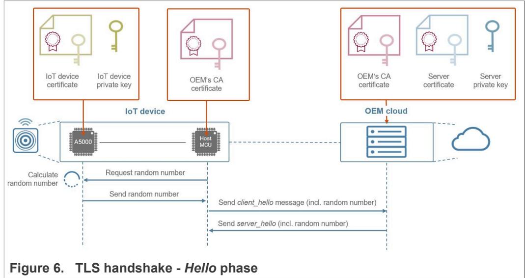
Figure 6. TLS handshake - Hello phase
