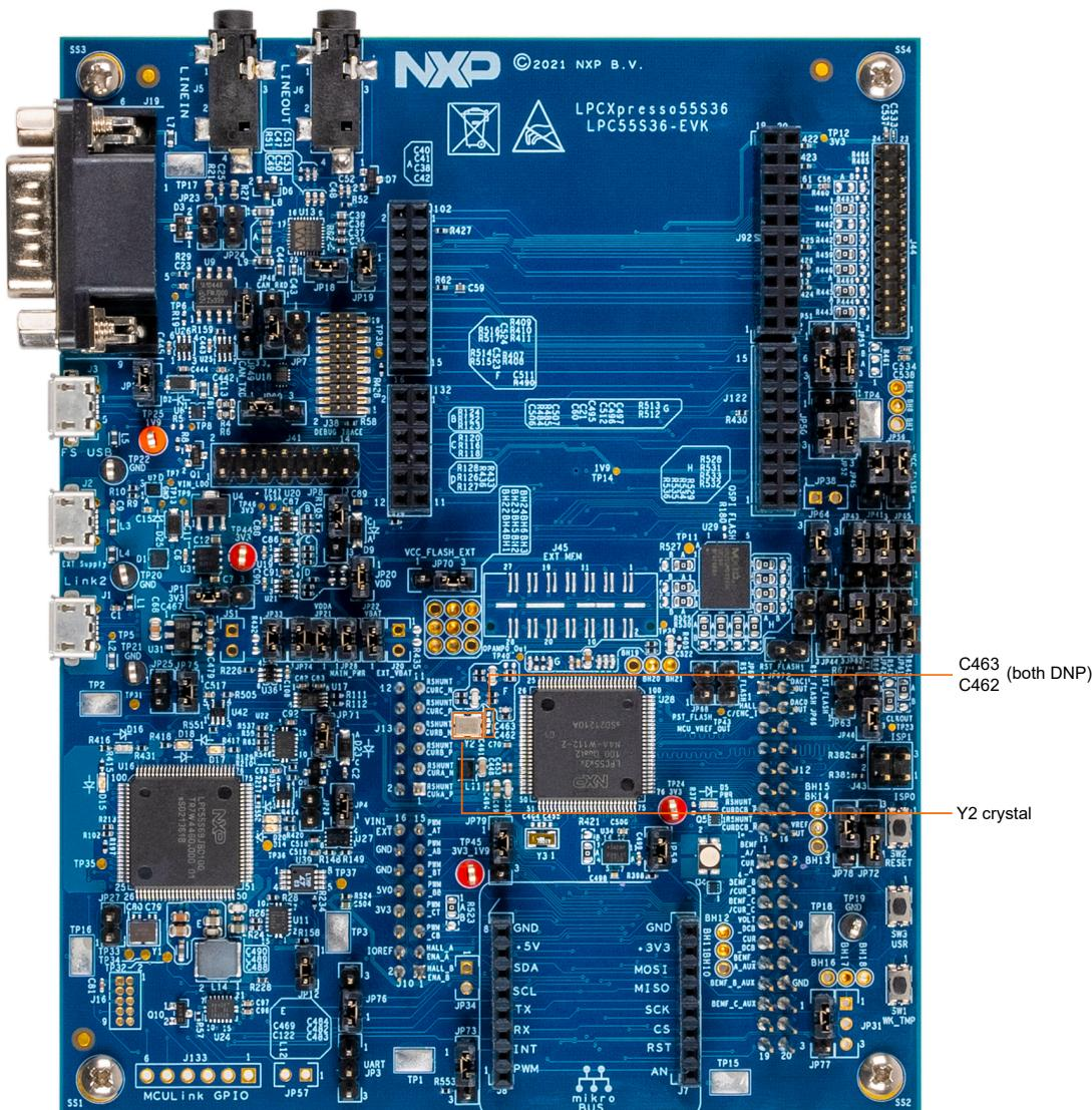
Figure 1. Optional components in LPCXpresso55S36 board
