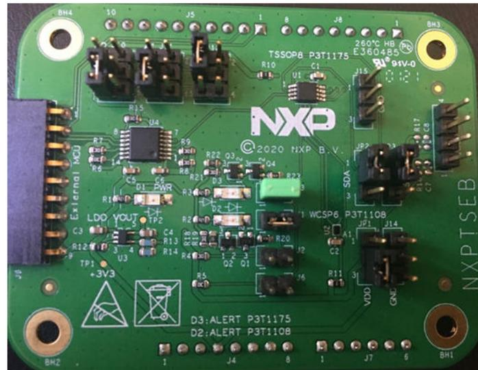
Figure 3. NXP P3T11xx Temperature Module
