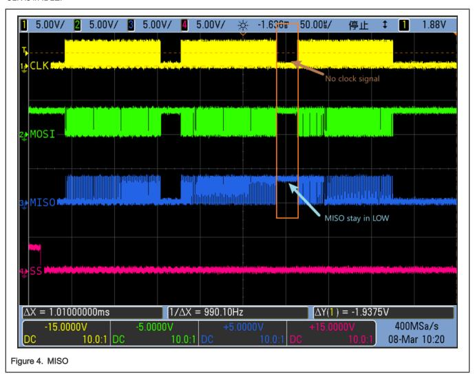
From description of ECSPI in datasheet, when SS is active, there is no requirement on MISO signal level.
