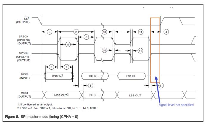
So this is not an issue here. ECSPI is able to guarantee that the data is sampled correctly.
