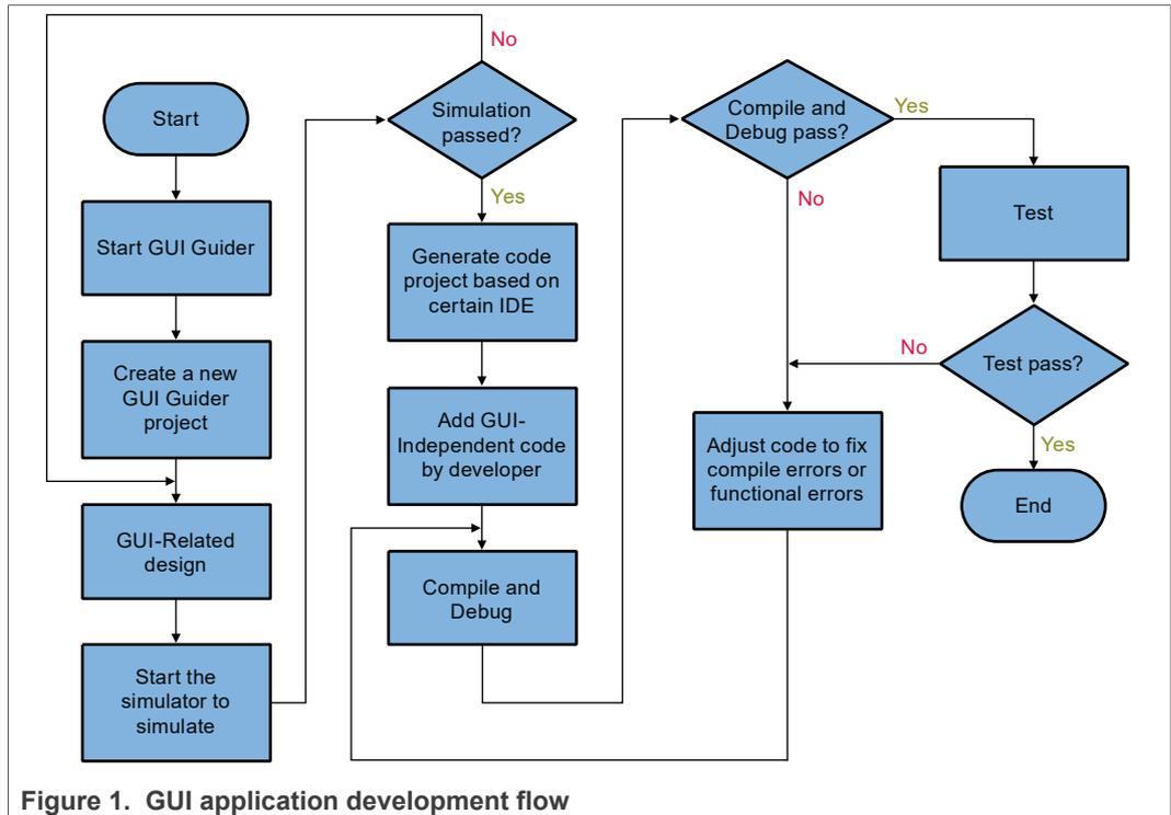
As shown in [Figure 1](#), after completing the design, it is recommended to perform a simulation to verify whether the simulation results are as expected or not. If the simulation is successful and as expected, the code can be generated. Otherwise, continue to adjust the design.
