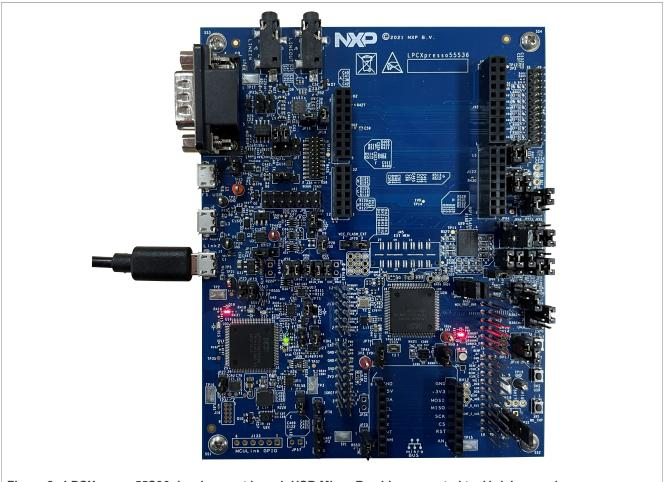
Figure 2. LPCXpresso55S36 development board; USB Micro-B cable connected to J1 debug probe
