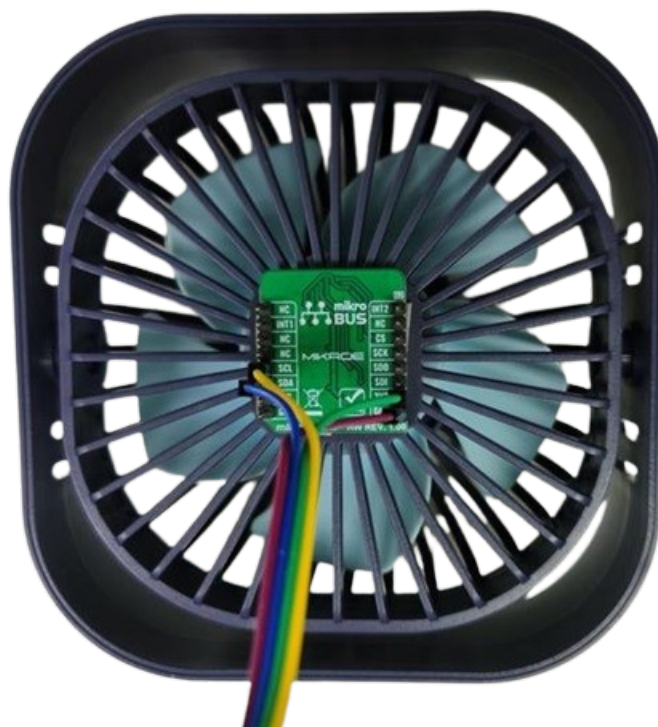
Figure 4. Mount the accelerator sensor on the FAN
