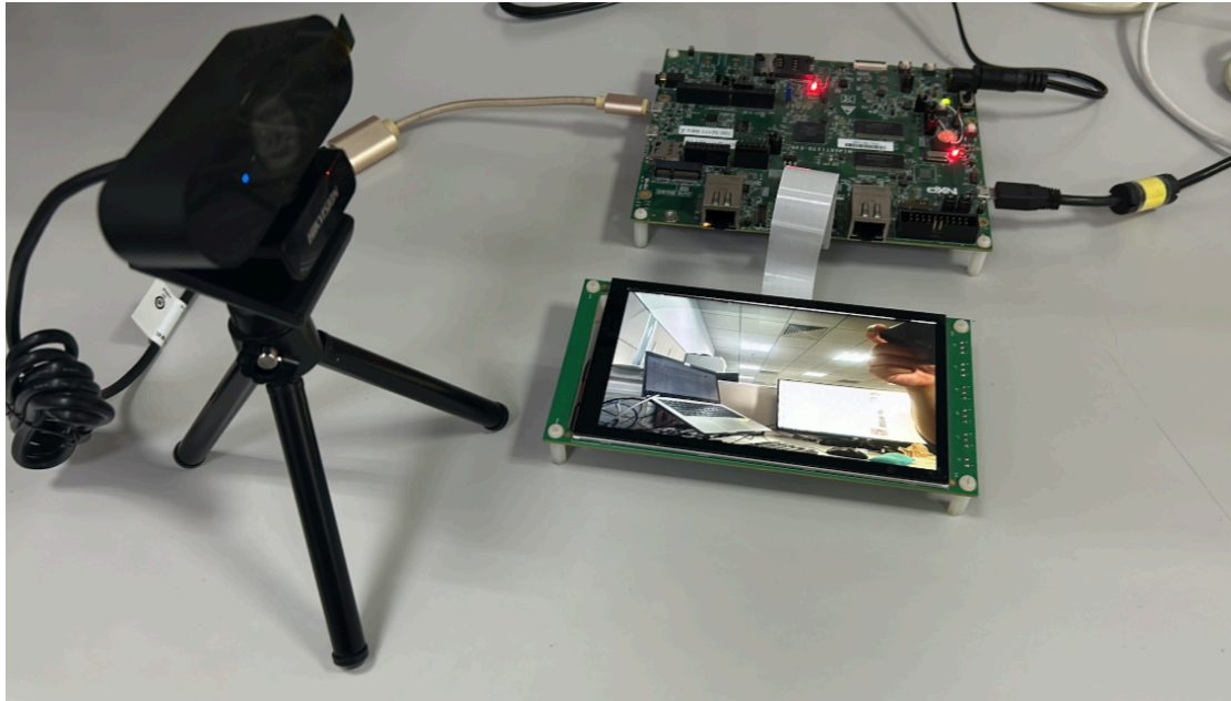
Figure 1. Connect USB camera and show picture on LCD panel using i.MX RT1170
