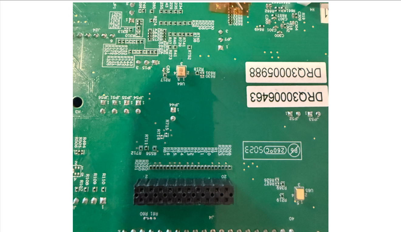
Figure 4. J53 header mounted at the bottom of the MIMXRT700-EVK board
