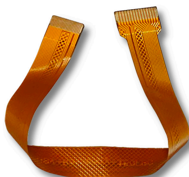
Figure 8. 22 pin (0.5 mm pitch) to 15 pin (1 mm pitch) FPC cable
