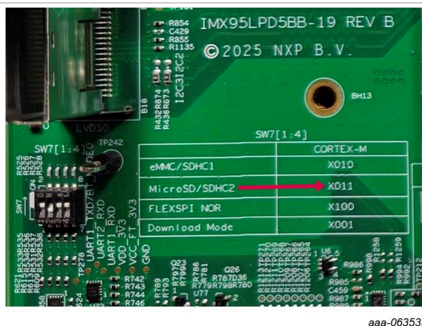
Figure 11. IMX95LPD5EVK-19 boot switch set to microSD/SDHC2 mode 1011 on SW7
