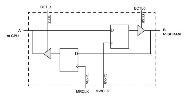
Figure 21. SDRAM Data Path Element
