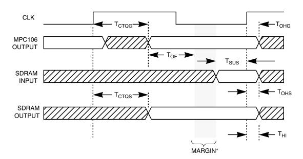
**Note:** The timing gap 'Margin' is the total allowance for errors due to system noise, clock jitter, clock skew and a host of other problems. The greater the margin, the greater the reliability and robustness of the SDRAM memory system.
