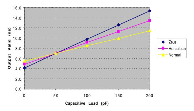
Figure 4. MPC106 83 MHz Output Valid Derating
