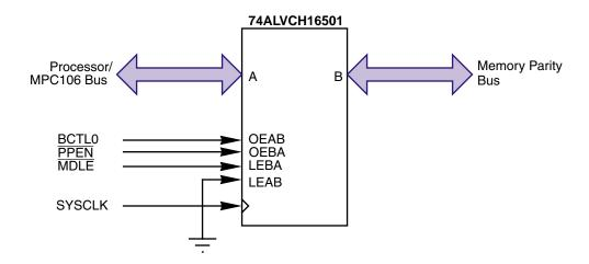
Figure 22. SDRAM Parity Bus
