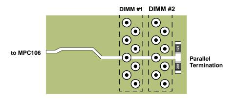
Figure 24. Parallel Termination Routing
