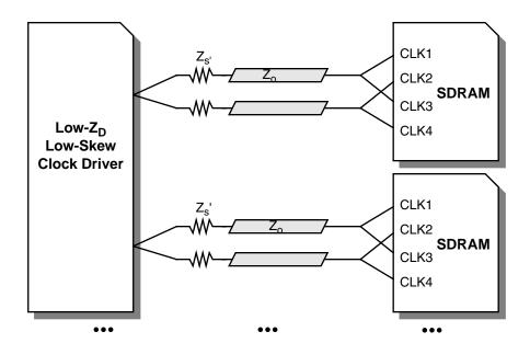
Figure 16. Multiply Shared Clock Architecture
