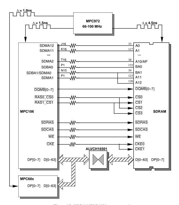
Figure 25. MPC106/SDRAM Interconnection
