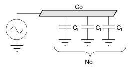
Figure 7. Distributed Capacitance
