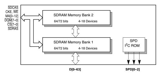
Figure 5. Typical SDRAM Module Block Diagram
