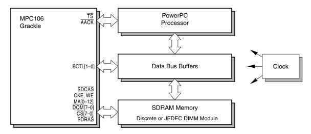
Figure 1. Typical SDRAM System Block Diagram
