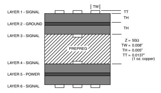
Figure 6. Typical PCB Stackup Diagram
