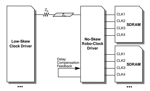
Figure 14. Distributed Clock Architecture
