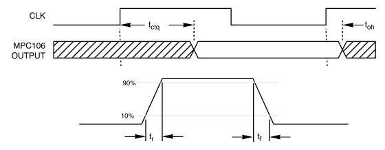
Figure 3. MPC106 Timing Parameters
