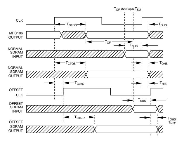
Figure 19. MPC106 Offset Clock Timing Diagram
