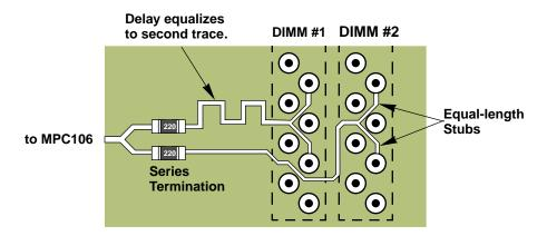
Figure 23. Series Termination Routing
