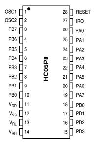
Figure 5. HC05P8 Pinout
