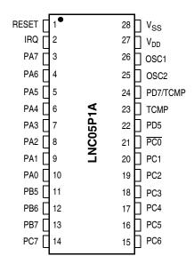
Figure 3. LNC05P1A Pinout
