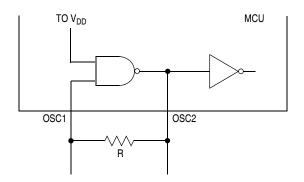
Figure 1. RC Oscillator Circuit Diagram
