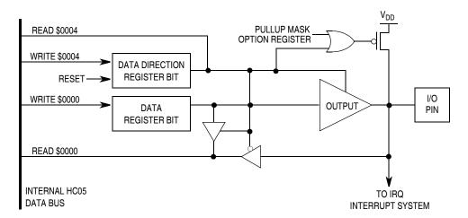
Figure 7. Port A I/O and Interrupt Circuitry
