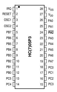
Figure 4. HC705P3 Pinout
