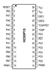
Figure 6. HC05P15 Pinout
