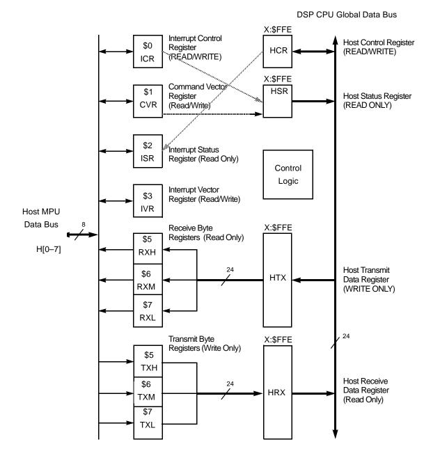
Figure 4. DSP56002 Host Block Diagram
