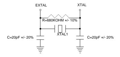
Figure 2. DSP56002 Fundamental Frequency Crystal Oscillator Circuit
