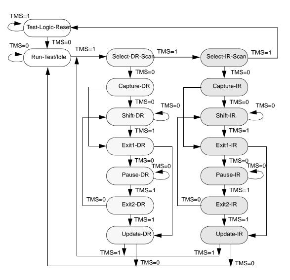
Figure 7. TAP Controller State Machine
