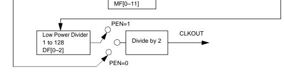
Figure 1. PLL Block Diagrams
