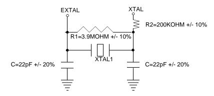
Figure 3. DSP56303 Fundamental Frequency Crystal Oscillator Circuit
