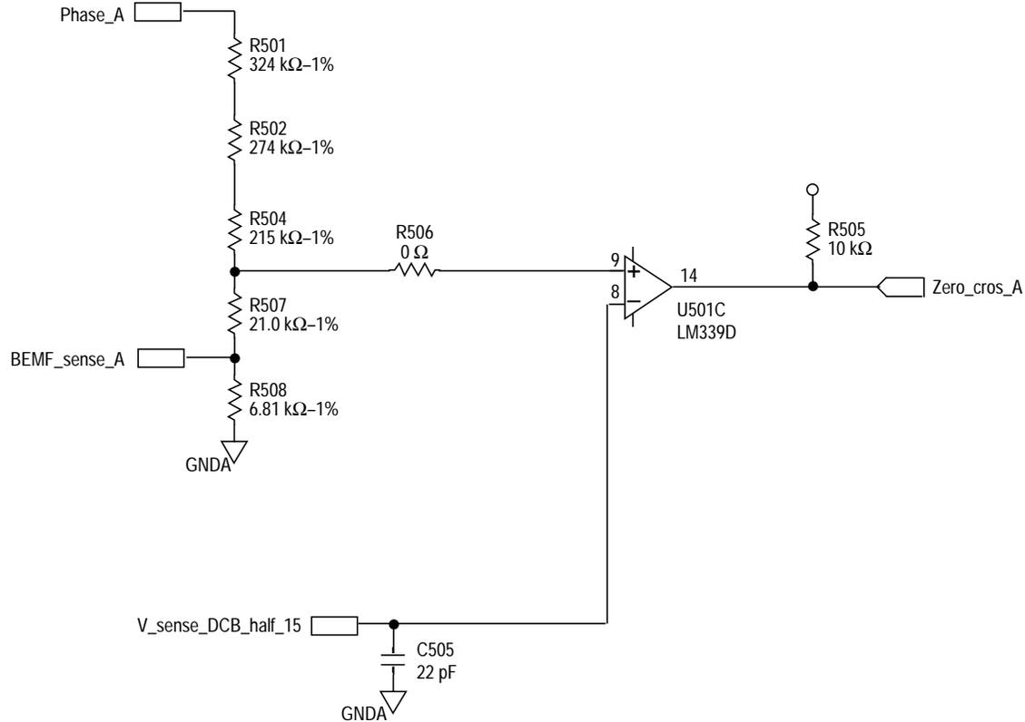
Figure 18. Back-EMF and Zero Cross Detection Schematic
