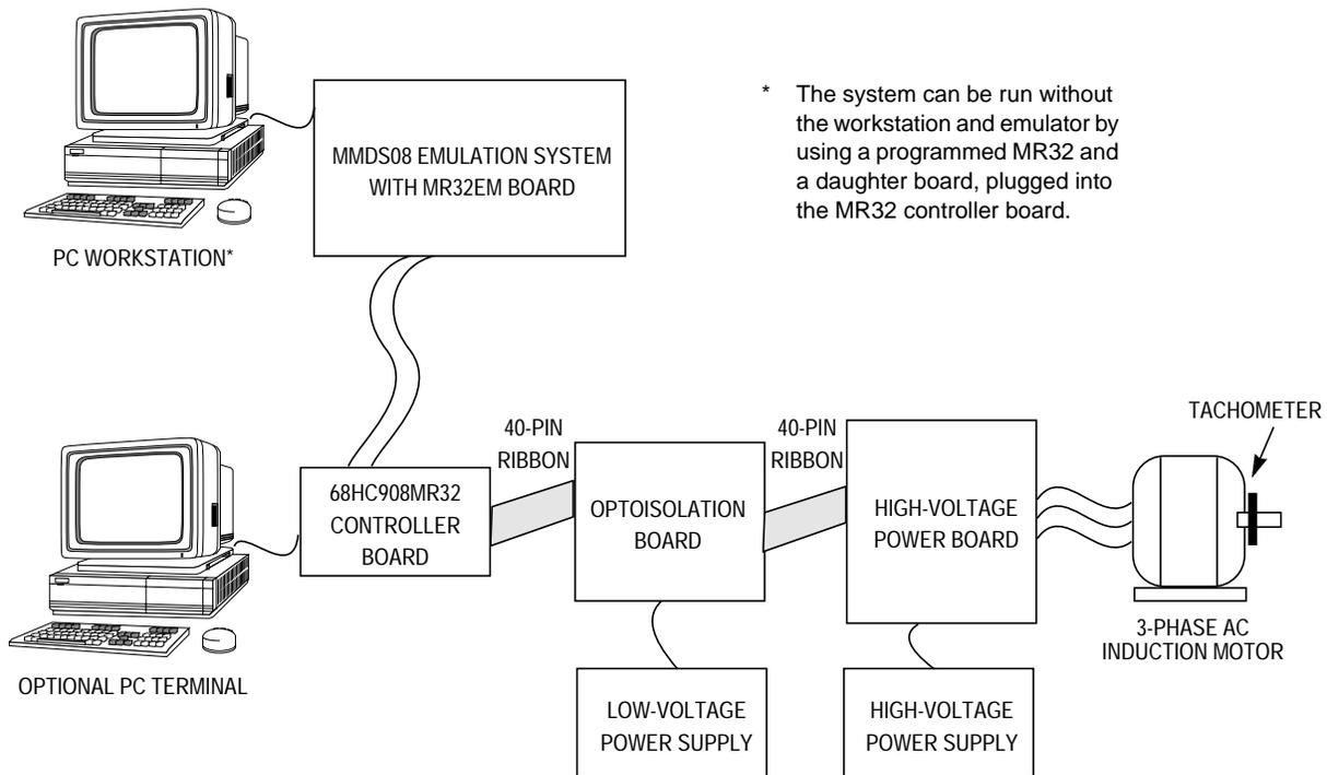
**Figure 19. 3-Phase Motor Control System Block Diagram**
