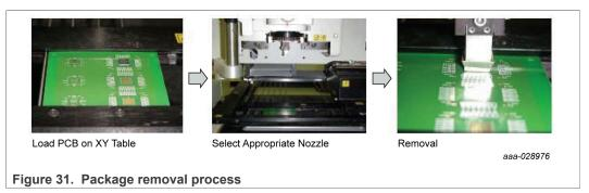
If the PCB is large, it is important to avoid bending of the printed circuit material due to thermal stress, so a bending prevention tool must be placed on the bottom of the printed circuit board, and a bottom heater installed (to allow heating of the entire printed circuit board, to raise work efficiency).
