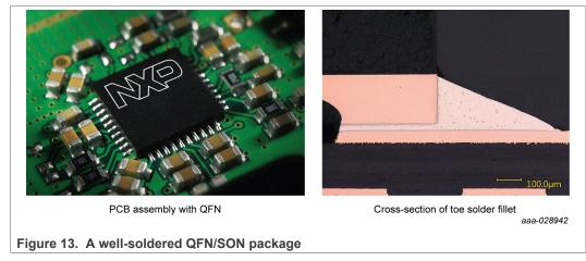
The cross-section picture in <u>Figure 13</u> shows the goal of a well-soldered QFN/SON terminal, void-free solder joint and a smooth solder fillet.
