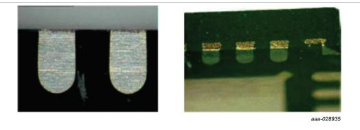
Figure 6. Fully-exposed terminal ends (package bottom and side view)
