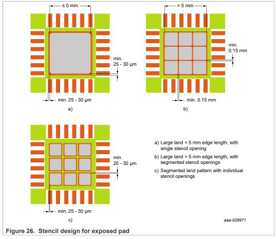
An array of smaller paste deposits for exposed pad land supports outgassing of the flux during reflow. Otherwise the evaporated flux is entrapped in the solder joint and creates large solder voids. Smaller QFN/SON packages can take advantage of this stencil design even for exposed pad size < 5 mm.
