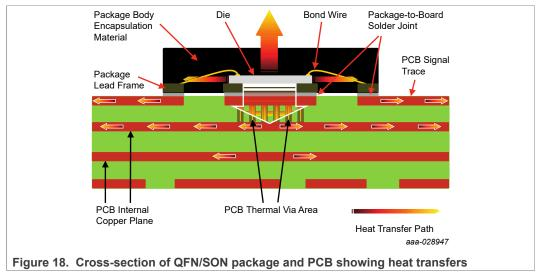
Although the land pattern design of the perimeter lands for exposed pad packages should be the same as that for non-thermally/electrically enhanced packages, extra
