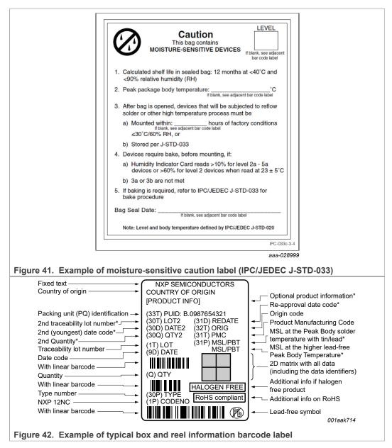
The MSL indicates the floor life of the component, its storage conditions, and handling precautions after the original container has been opened. The permissible time, from opening the moisture barrier bag until the final solder reflow process, that a component can remain outside the moisture barrier bag is a measure of the sensitivity of the component to ambient humidity.
