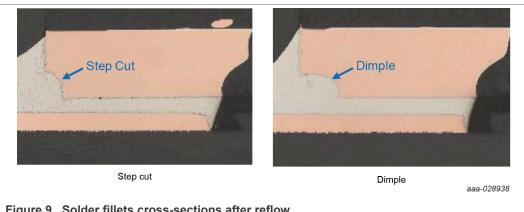
Figure 9. Solder fillets cross-sections after reflow
