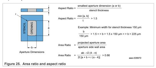
Maximum thermal/electrical performance requires that the exposed pad of the package is soldered to the land pattern on the PCB. The maximum aperture size of the stencil should not exceed > 5 mm on either side (Figure 26a). Larger openings should be subdivided into an array of smaller openings as shown in Figure 26b. The spacing between segments on the stencil should be 0.150 mm or more. Narrower spacing between segments can become a manufacturing issue.
