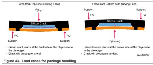
• Force F<sub>(Bottom)</sub> applied on package bottom side, where bending stress at the active die surface could exceeds silicon fracture strength
