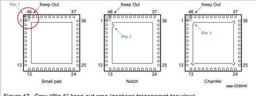
Figure 17. Gray "Pin 1" keep out area (package transparent top view)
