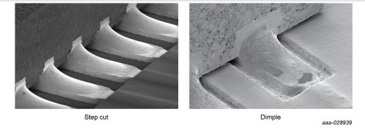
Figure 10. SEM Images of solder fillets cross-sections after reflow
