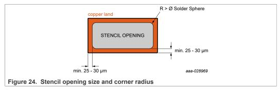
A minimum aperture size is needed to ensure the proper release of the solder paste during stencil printing (Figure 24). The area ratio and the aspect ratio between stencil opening and stencil thickness are used to determine the minimum dimensions, respectively.
