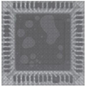
Not segmented exposed pad with large solder voids and terminals with shorts/bridging aaa-028975
