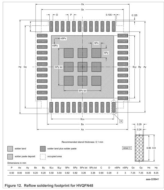
**Note:** This footprint is meant be used as guideline and a starting point for individual PCB designs. To achieve optimum assembly quality, the user must adapt the footprint to meet needs, assembly, and application environment.
