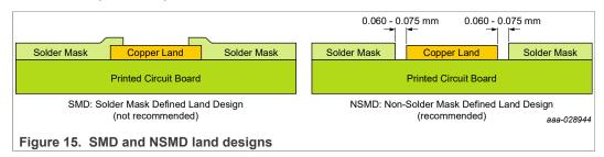
Each land should have its own solder mask opening with a web of solder mask between two adjacent leads (Figure 16). IPC-7351 recommends having at least 0.075 mm of web width to ensure adhesion to the PCB surface is sufficient. Minimum solder mask width will also depend on PCB manufacturer capabilities.
