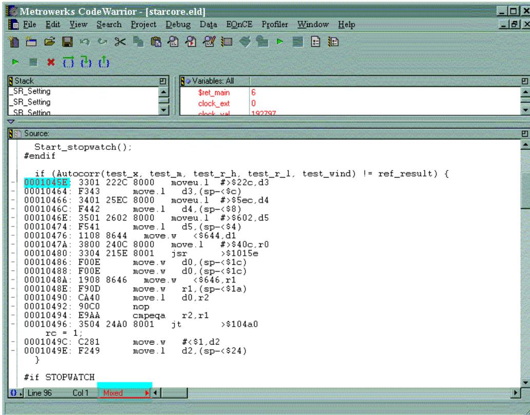
**Figure 4. Finding the Starting Address in Debugger**
