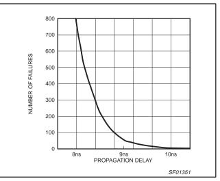
Figure 1. Exponential Decay of Failures
