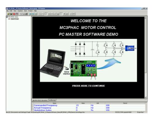
Figure 5. PC Master Software Application Workspace
