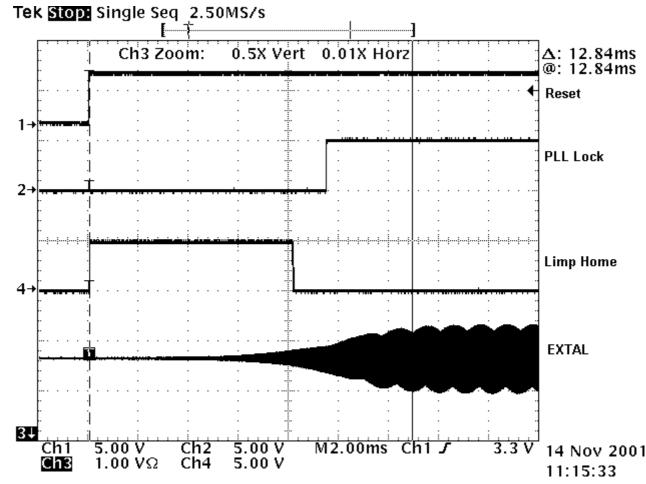
The trace shows that the time from the release of the Reset pin till PLL lock is about 9.5mS, far greater than the calculated 2.3mS. Even without the advantage of being able to observe the EXTAL signal, the Reset – PLL Lock measurement clearly indicates that the application has oscillator start-up issues which merit further investigation.
