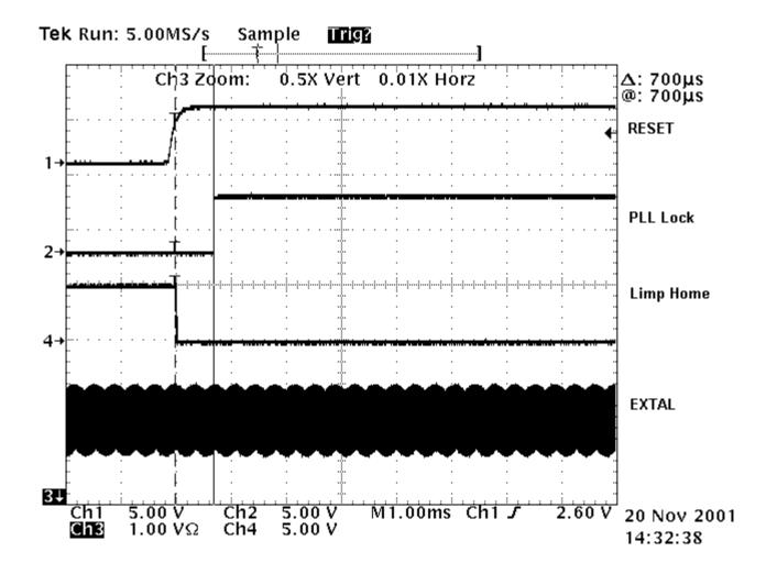
In this trace Reset has been held low externally for a sufficiently long time to allow the oscillator to become stable, and the internal 4096 cycle delay to be completed. Here the PLL achieves lock very quickly, in almost the exact time predicted by the PLL lock time calculation. This indicates that the oscillator start-up exhibits a good performance.
