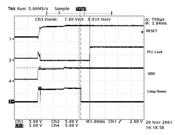
This trace shows where Limp Home Mode is de-asserted. We cannot tell from the scope trace whether Limp Home Mode was de-asserted either during or after the 4096 cycle delay. We can see from this trace that the PLL achieves lock 0.7mS after the MCU exits Limp Home Mode. This suggests that the oscillator signal at EXTAL was stable when Limp Home Mode was de-asserted, as the PLL Lock time was estimated at 0.74mS.
