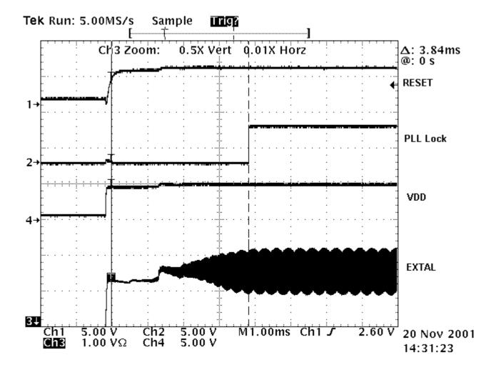
In this scope trace, Reset is released almost immediately after VDD. The scope trace clearly shows that the oscillator has not started when Reset is released, thus the MCU is in Limp Home Mode.
