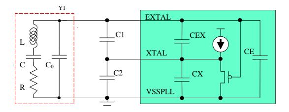
In this instance  $Z_0$ , = C\_' = C\_ + CE,  $Z_1$  = C\_' = C\_ + CEX, and  $Z_2$  = C\_' = C\_ + CX.
