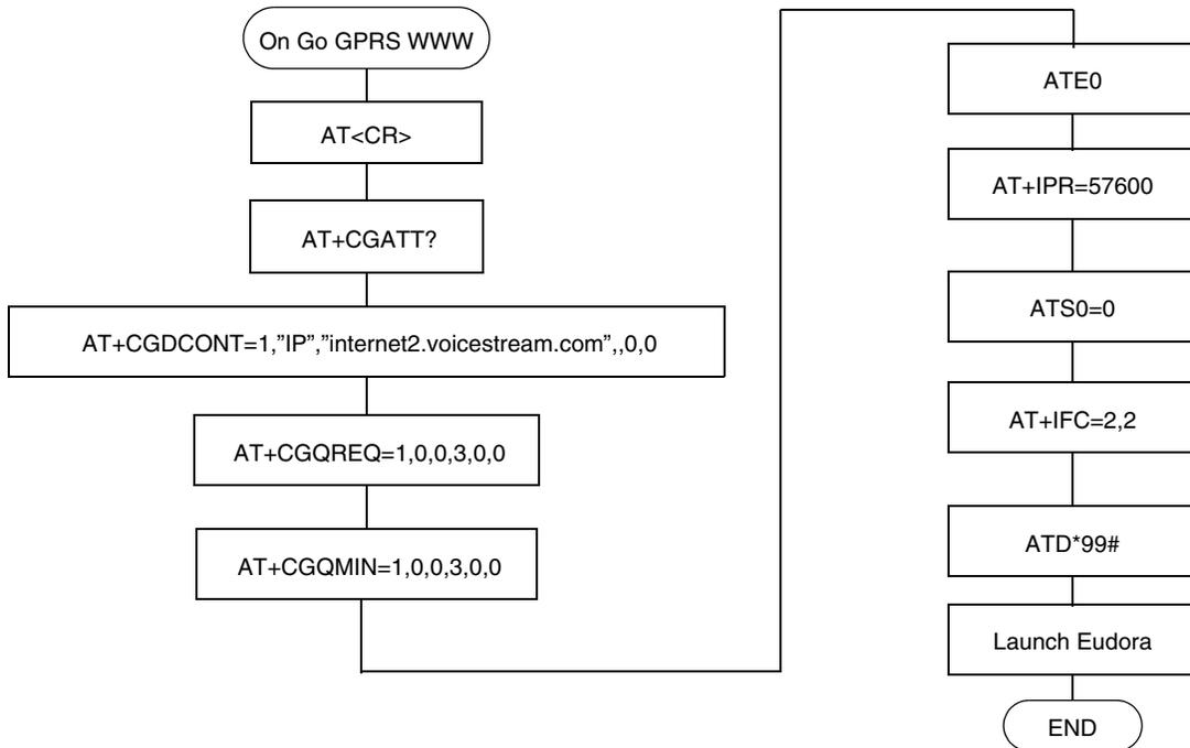
Figure 3. GPRS Initialization Flow Chart
