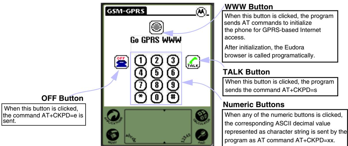
Figure 1. *GSM-GPRS* Application GUI
