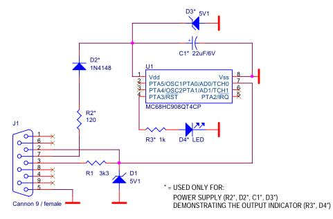
Figure 4. Basic Demo Schematic
