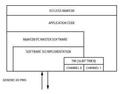
Figure 3. M68HC08 PC Master Software for M68HC08 MCUs That Don't Have SCI
