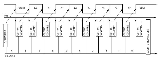
Figure 6. Output Compare Driven Transmission Time Chart
