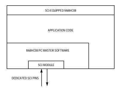
Figure 2. Traditional (SCI-Equipped) M68HC08 PC Master Software
