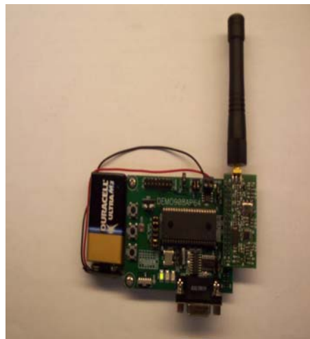
Figure 2. MC68HC908AP64 and Romeo2 RF Module
