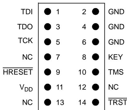
**Figure 5.** 14-Pin Header for JTAG/Emulator Interface
