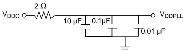
Figure 1. PLL Power Supply Filter Circuits
