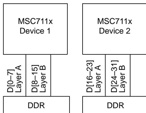
**Figure 4.** Example of Data Routing For Multiple DSPs
