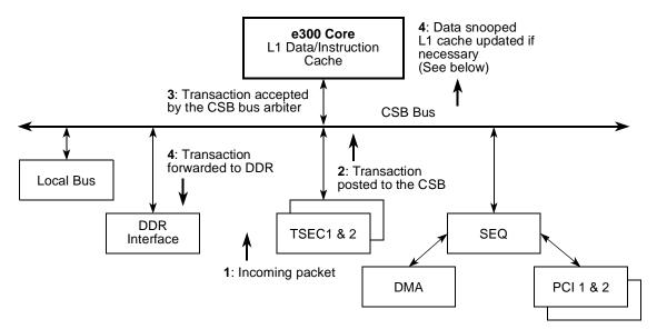
Figure 11. Global Transaction Example (Received Ethernet Frames are Snooped)
