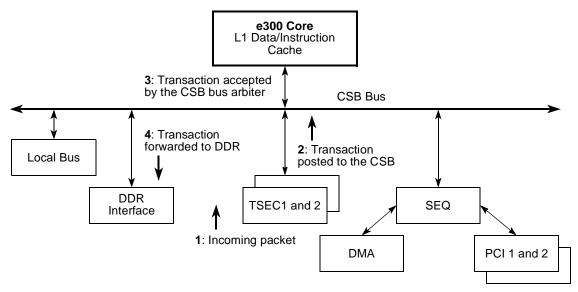
Figure 10. Non-Global Transaction Example (Received Ethernet Frames are Not Snooped)
