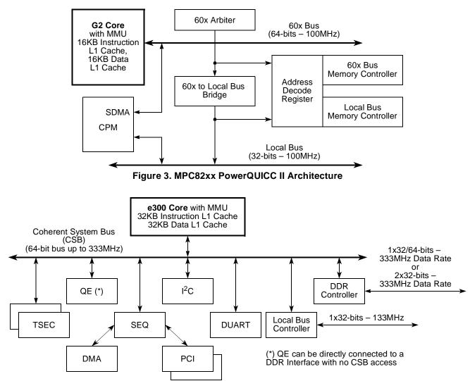
Figure 4. MPC83xxPowerQUICC II Pro Architecture
