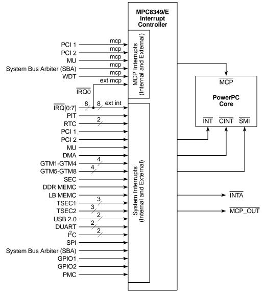
Figure 15. MPC83xx IPIC Structure
