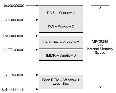
Figure 8. MPC8349 Memory Map Windows After Configuration
