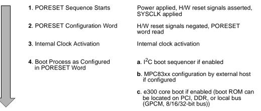
Figure 12. MPC83xx PORESET Sequence
