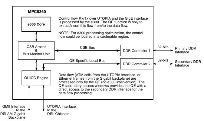
Figure 9. Example Usage of the QUICC Engine Secondary DDR Interface
