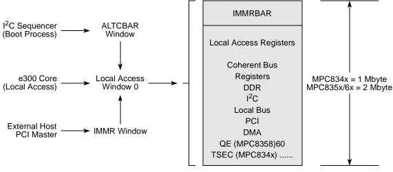
Figure 13. MPC83xx Internal Configuration Masters
