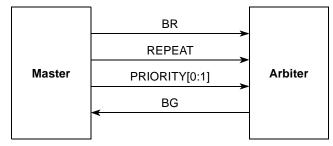
Figure 5. CSB Master Arbitration Signals
