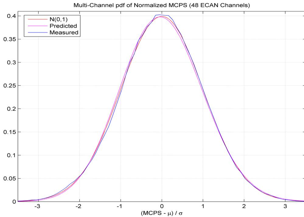
**Figure 4.** Estimated PDF Measurement of 48 Echo Canceller Channels Versus Theoretical Predictions
