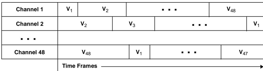
Figure 2. Echo Canceller Multi-Channel Loading Scheme
