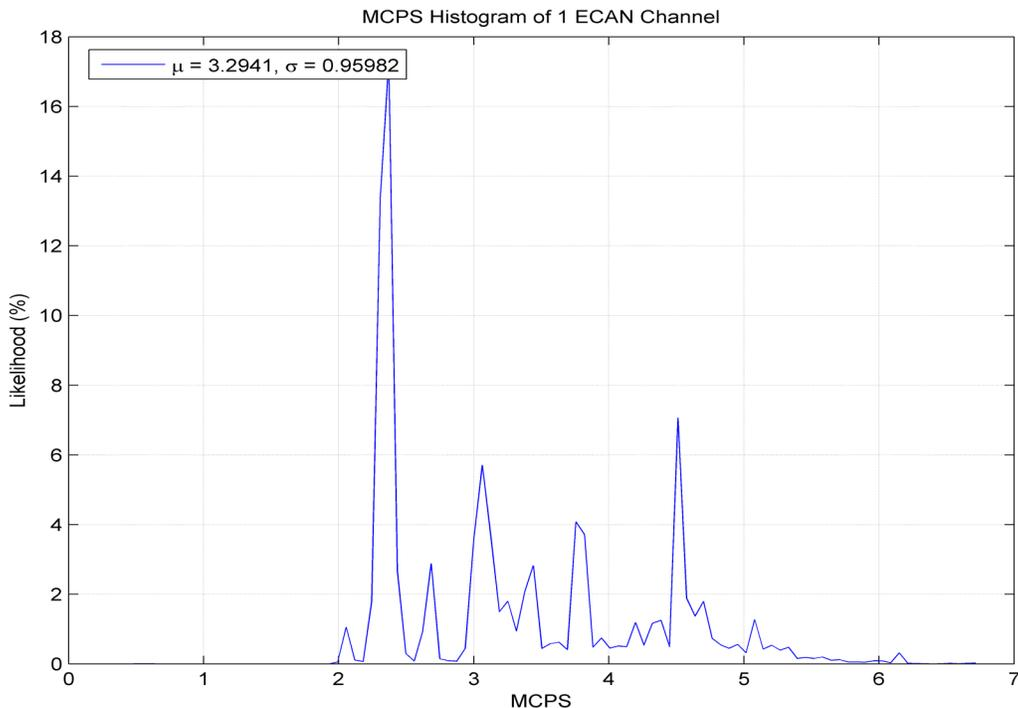
Figure 1. MCPS Histogram of a Single Echo Canceller Channel
