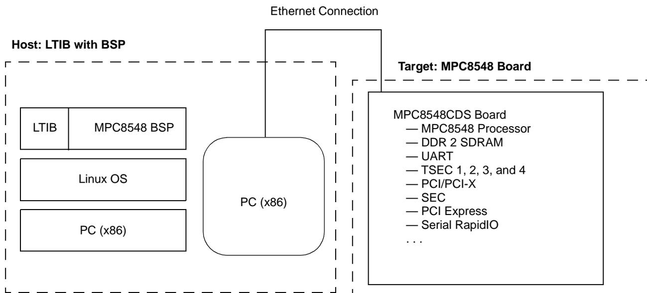
Figure 1. MPC8548E BSP on x86 PC Running Linux OS
