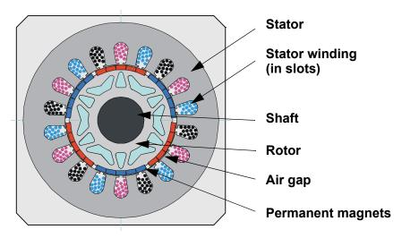
Figure 2. Permanent Magnet AC Machine - Cross Section
