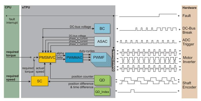
Figure 13. Block Diagram of eTPU Processing
