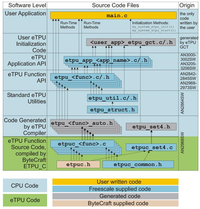
Figure 9. eTPU Project Structure
