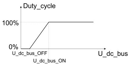
Figure 20. PWM Mode of the Break Controller Function
