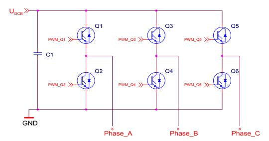
Figure 3. 3-Phase Power Stage
