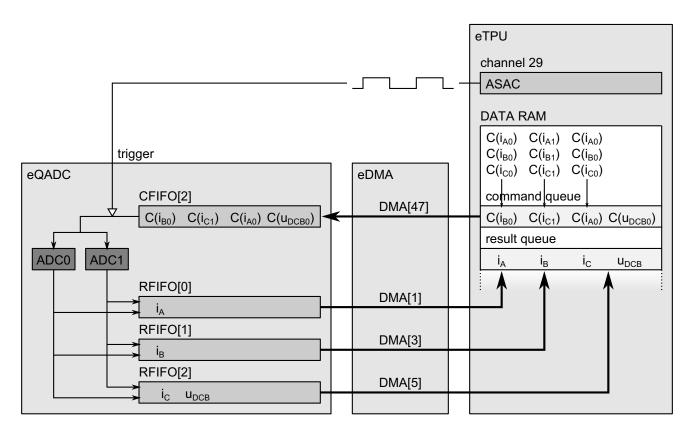
Figure 16. Cooperation of eTPU, eDMA and eQADC modules
