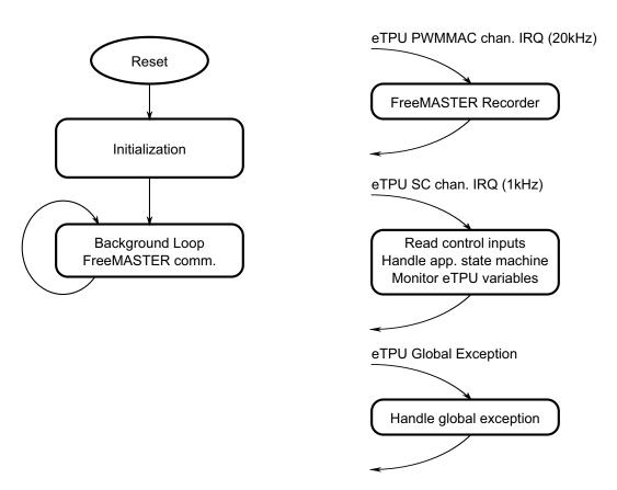
Figure 10. CPU Software Flowchart
