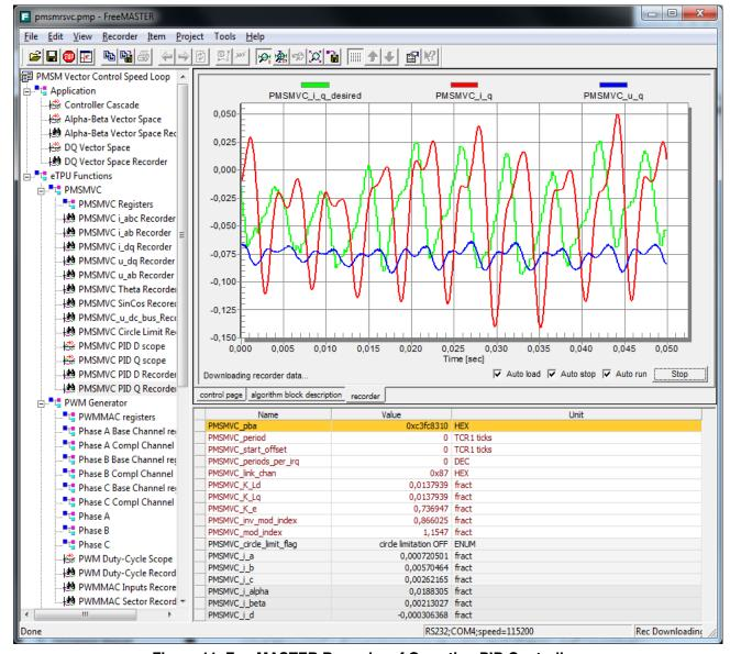
Figure 11. FreeMASTER Recorder of Q-portion PID Controller
