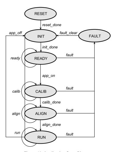
Figure 12. Application State Diagram
