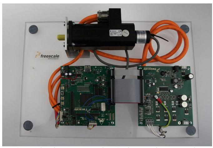
Figure 1. MPC5554 Controller Board, Power Stage with MC33937, and TGT2-0032-30-24 PMSM
