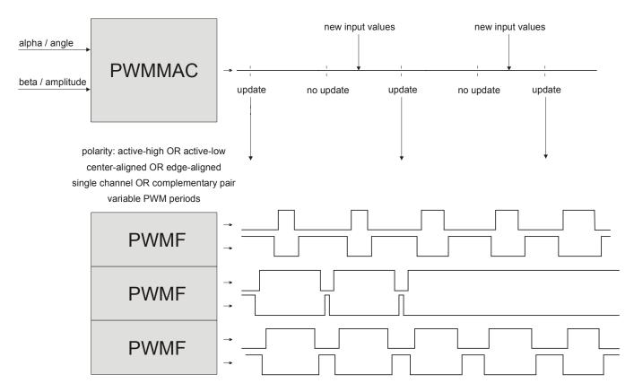
Figure 14. Functionality of PWMMAC+PWMF
