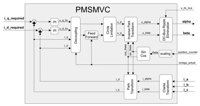
Figure 4. PMSM Vector Control Current Loop Block Diagram
