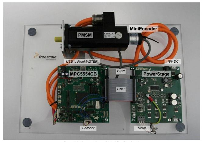
**Figure 8. Connection of Application Parts**
