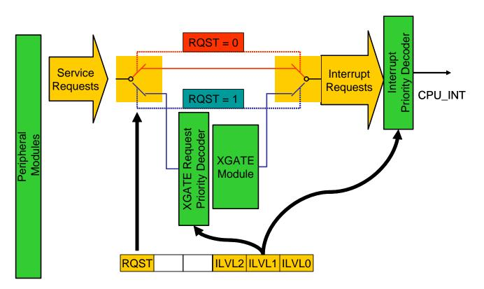
Figure 1. Interrupt Paths Using CPU or XGATE
