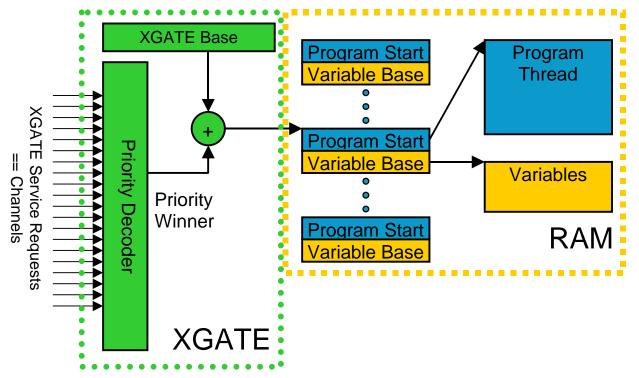
Figure 9. Vector and Data Pointer for XGATE Routines
