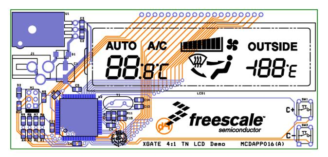
Figure 8. PCB Demo Board where the XGATE Controls the LCD Panel Directly
