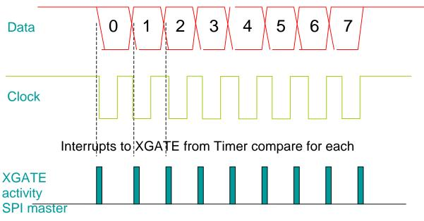
Figure 6. Serial Peripheral Interface (SPI) Master
