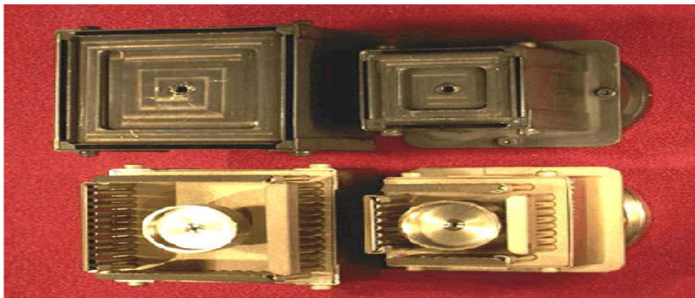
Figure 6. Shell Type Preheat Tool/Vacuum Pick-up Tool
