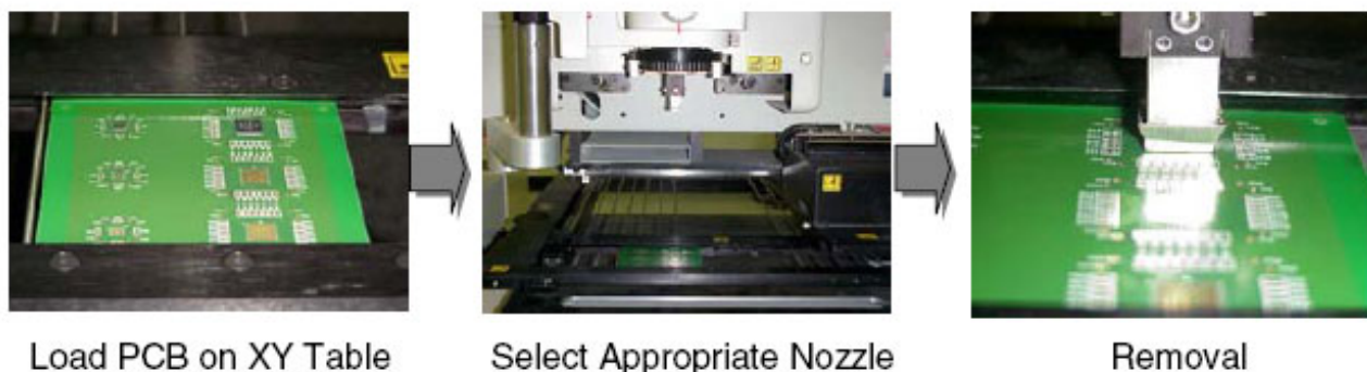
Figure 4. Typical Package Rework Station and Process
