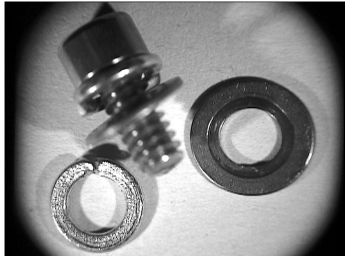
Figure 5. Mounting Hardware: Socket Head Cap Screw, Split and Flat Washers
