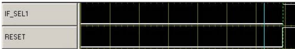
Figure 6. Fail Case 2 — MFR4300 Switches to the TXD_BG Output Function after Very Short Delay
