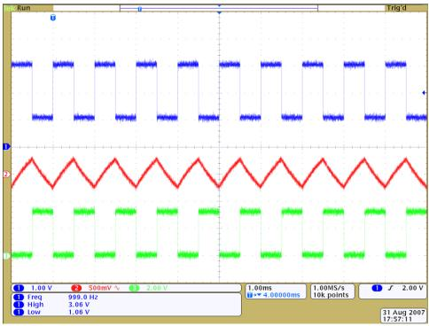
Figure 11. DC Offset Elimination Waveforms
