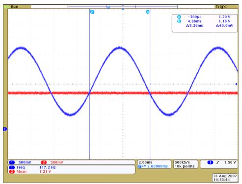
Figure 7. Pulse-Width Measurement Waveform—1.2 V Reference
