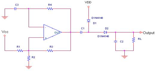
Figure 12. Voltage Doubler Circuit
