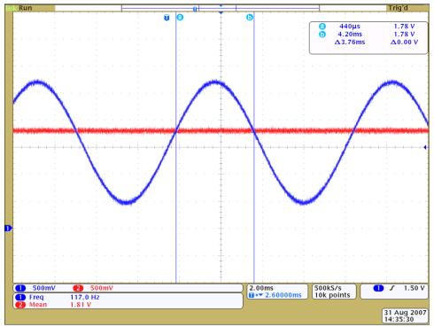
Figure 8. Pulse-Width Measurement Waveform—1.8 V Reference
