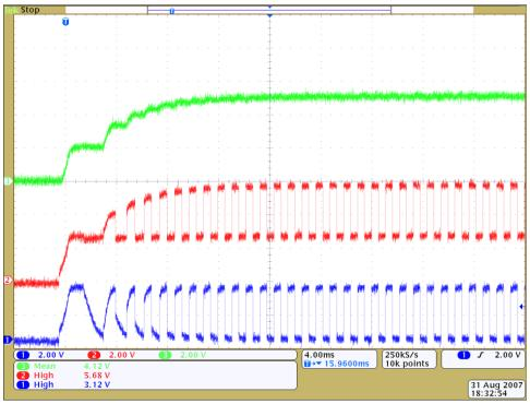
Figure 13. Voltage Doubler Waveforms
