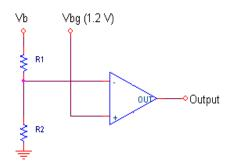
Figure 2. Voltage Monitoring Circuit Using Internal Reference
