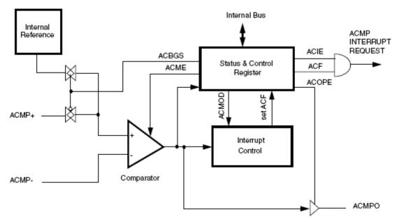
Figure 1. Analog Comparator Module Block Diagram
