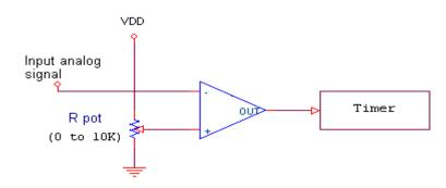
Figure 6. Pulse Width Measurement Circuit
