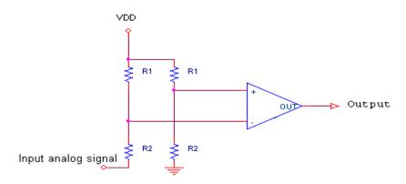
Figure 14. Zero Crossing Detector Circuit
