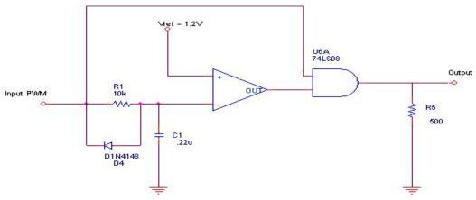
Figure 16. Auto Turn Off Circuit
