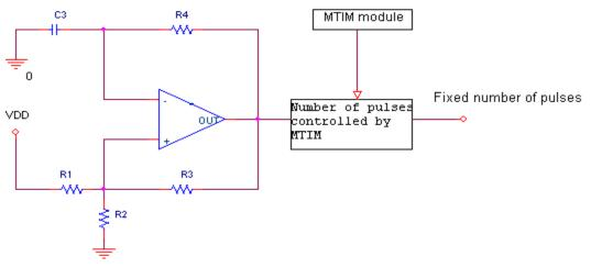
Figure 19. Fixed Number Pulse Generator Circuit
