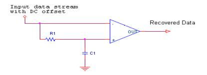
Figure 10. DC Offset Elimination Circuit
