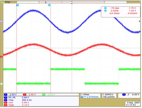
Figure 15. Zero Crossing Detector Waveforms
