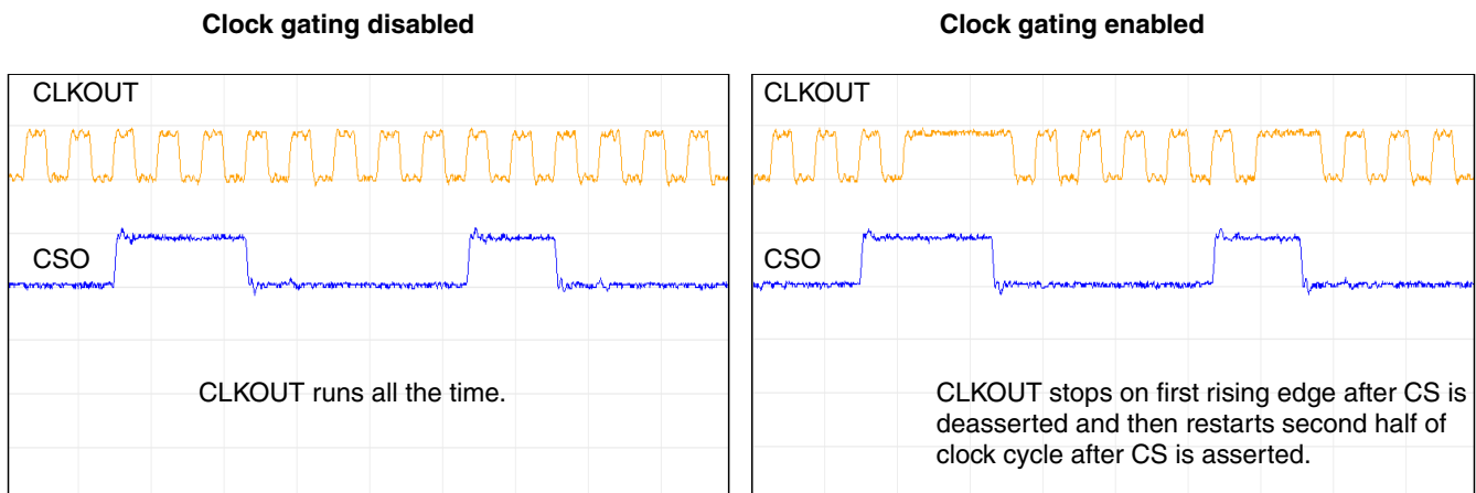
Figure 12. EBI Automatic Clock Gating (Clkout, CS)
