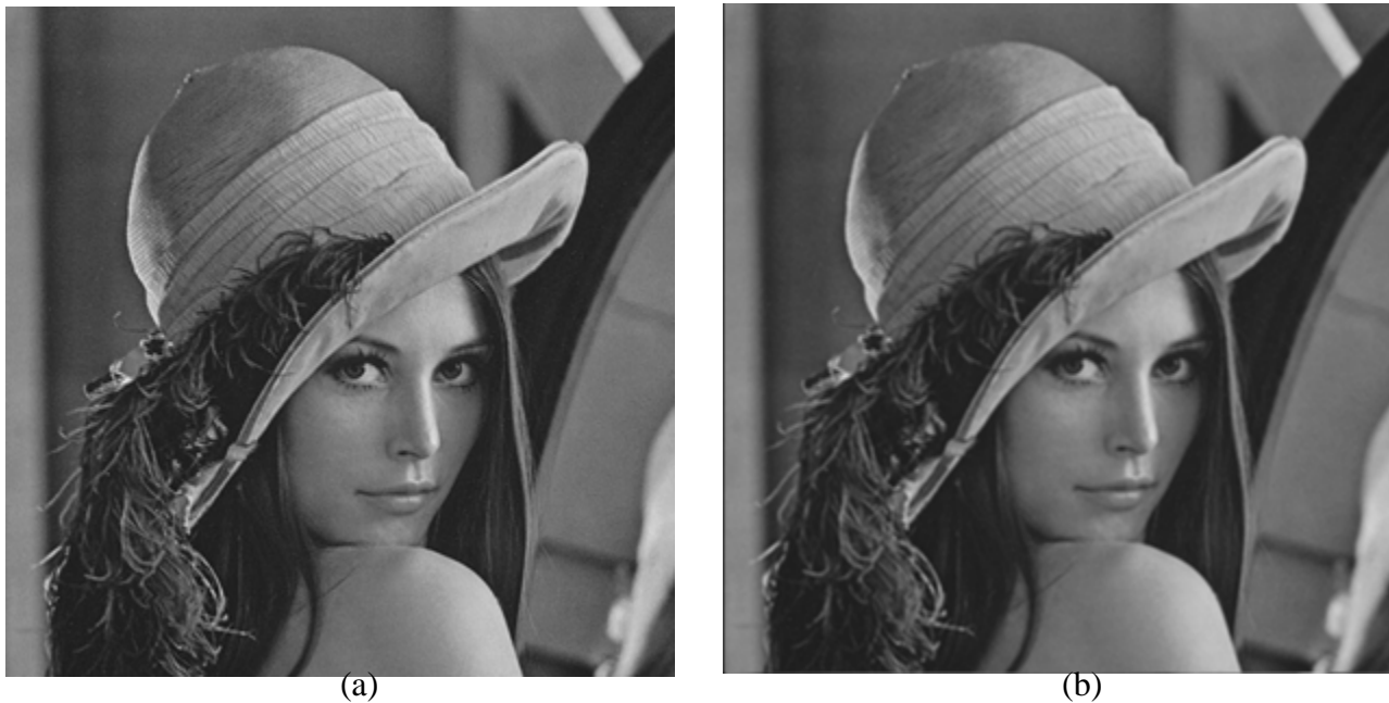
(a) Input image of size (rows x cold) (b) Image filtered using an average mask
