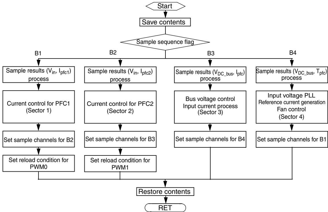
Figure 13. ADC ISR Flowchart
