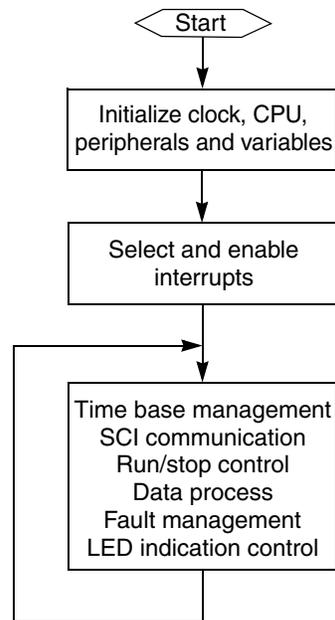
**Figure 11. Main Loop Flowchart**
