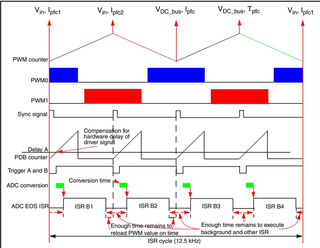
Figure 12. ADC Interrupt Control Sequence Diagram
