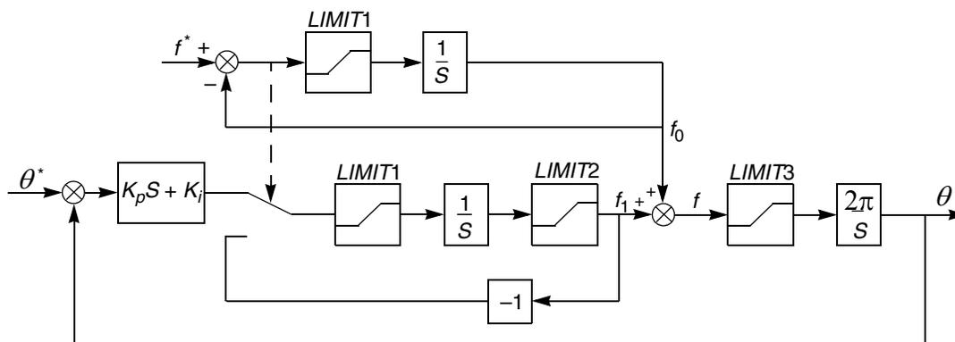
Figure 14. Input Voltage PLL Control Block Diagram
