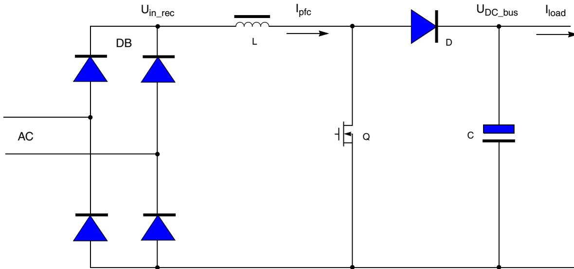
Figure 1. Single-Phase Boost PFC Converter Topology
