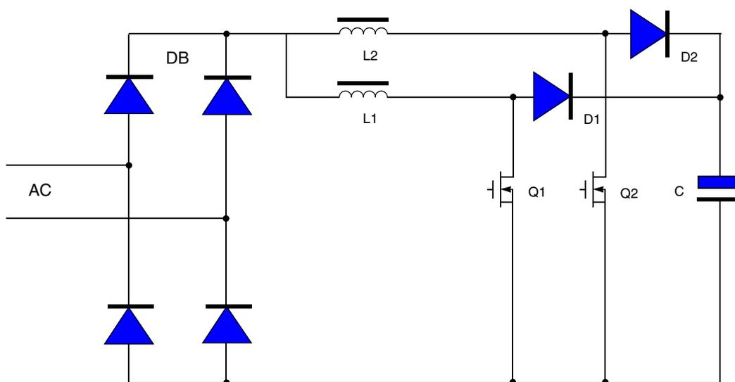
Figure 8. Main Power Topology Circuit
