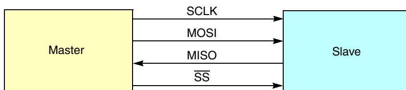
Figure 2. Single master, single slave SPI implementation
