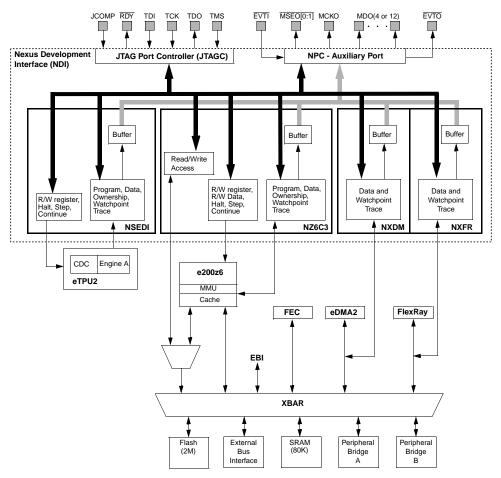
Figure 1. Typical MPC5500 Nexus Development Interface (MPC5567 shown)
