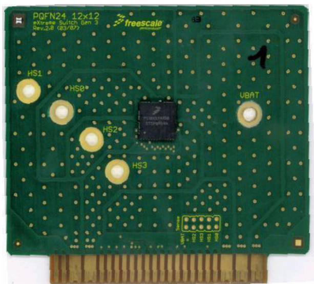
Figure 6. PCB #2 (coupon Board; High Thermal Conductivity) with eXtreme Switch Mounted
