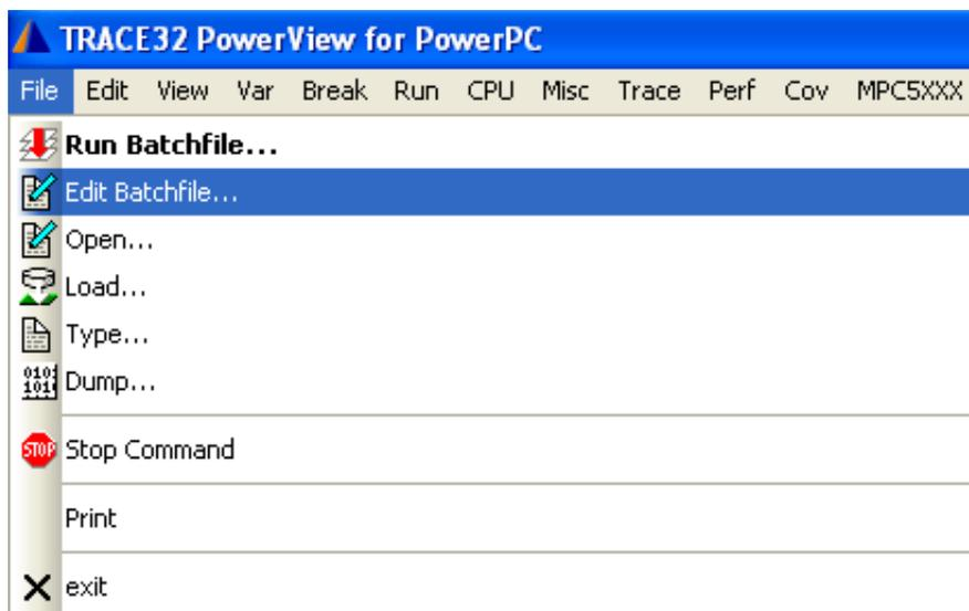
**Figure 2. Loading script file with Trace32 debugger**
