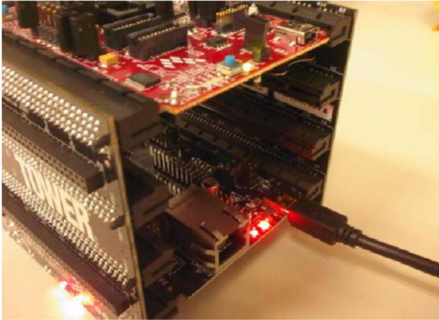
**Figure 22. Connecting TWR-SER USB cable**
