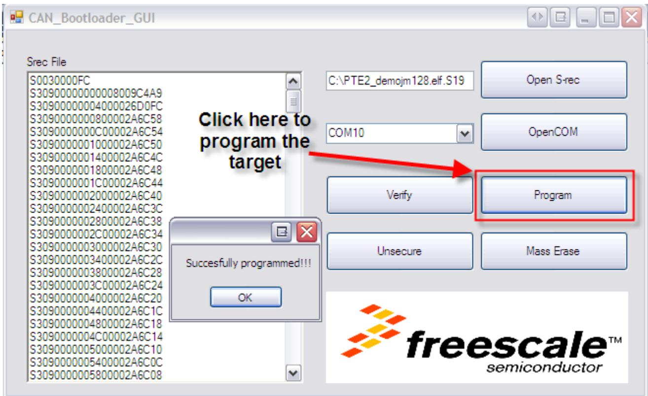
**Figure 13. Flash target**
