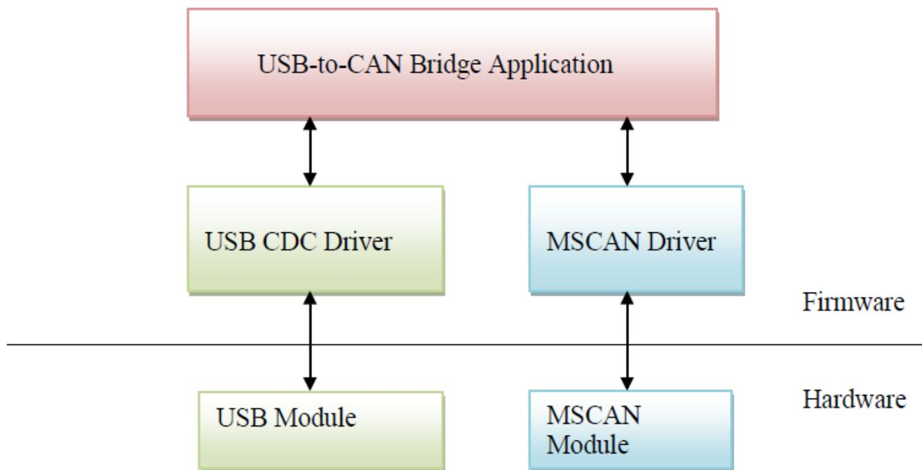
Figure 5. USB-to-CAN architecture
