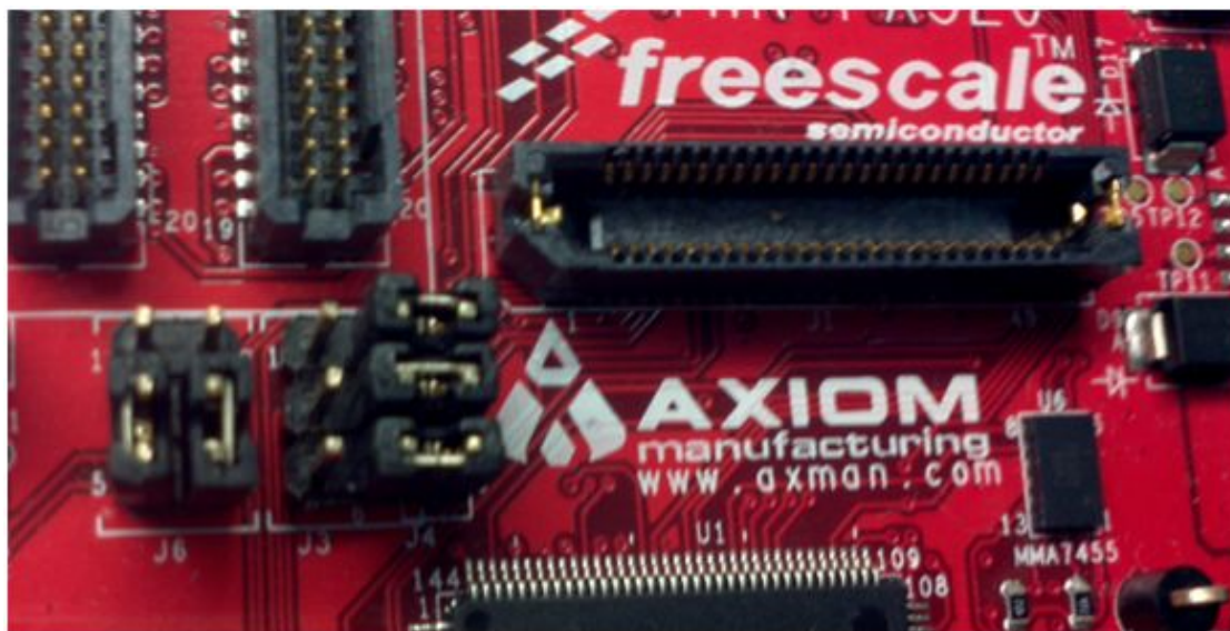
Figure 10. Default jumper configuration
