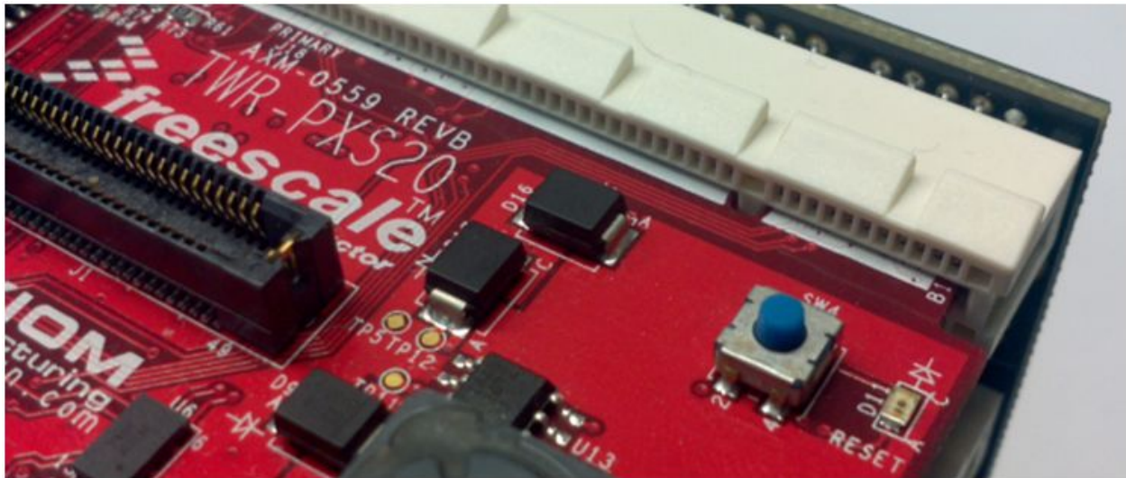
Figure 9. TWR-PXS20 RESET button
