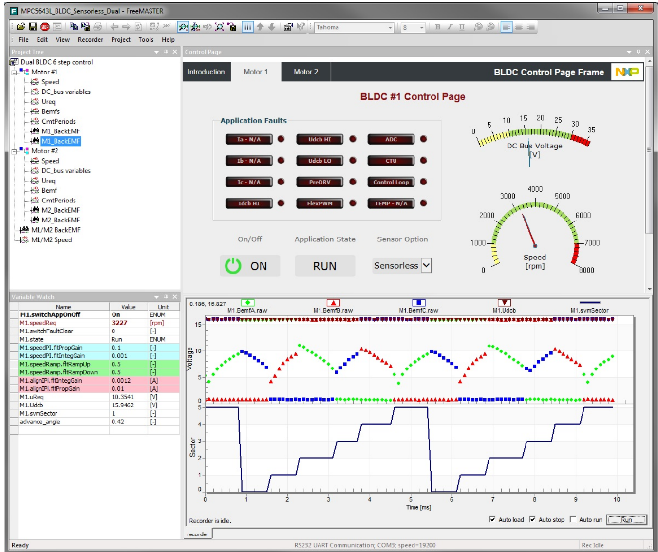
Figure 15. FreeMASTER control page for controlling the application
