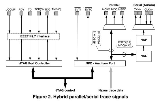
3. A lane consists of two signals, a positive signal and a negative signal.
