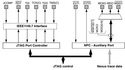
Figure 1. Parallel trace signals
