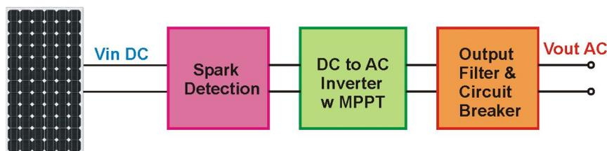
**Figure 2. Microinverter topology**
