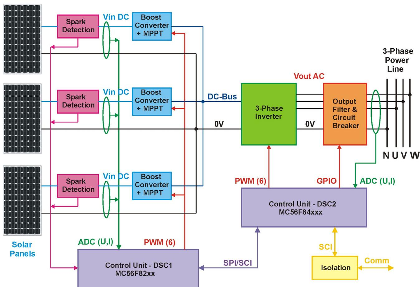
**Figure 4. Large three-phase inverter**
