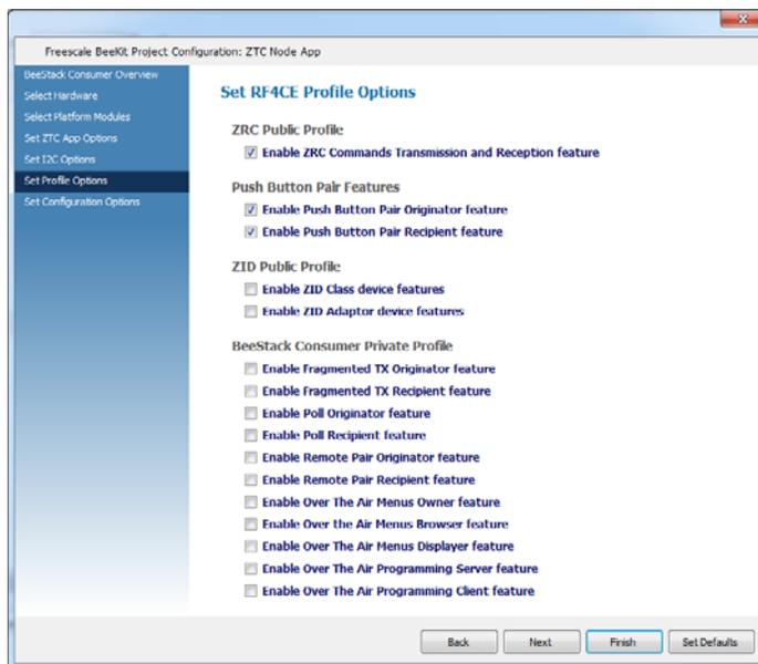
**Figure 9. Enabling ZRC commands and profile specific features**
