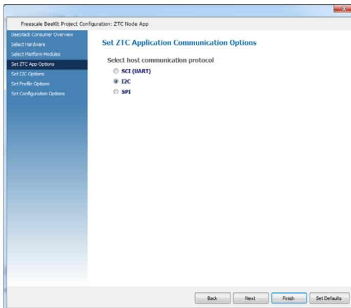
**Figure 8. Selecting the I2C BlackBox communication protocol**
