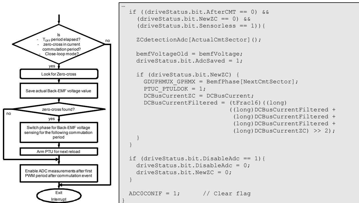
Figure 19. Commutation transients processing
