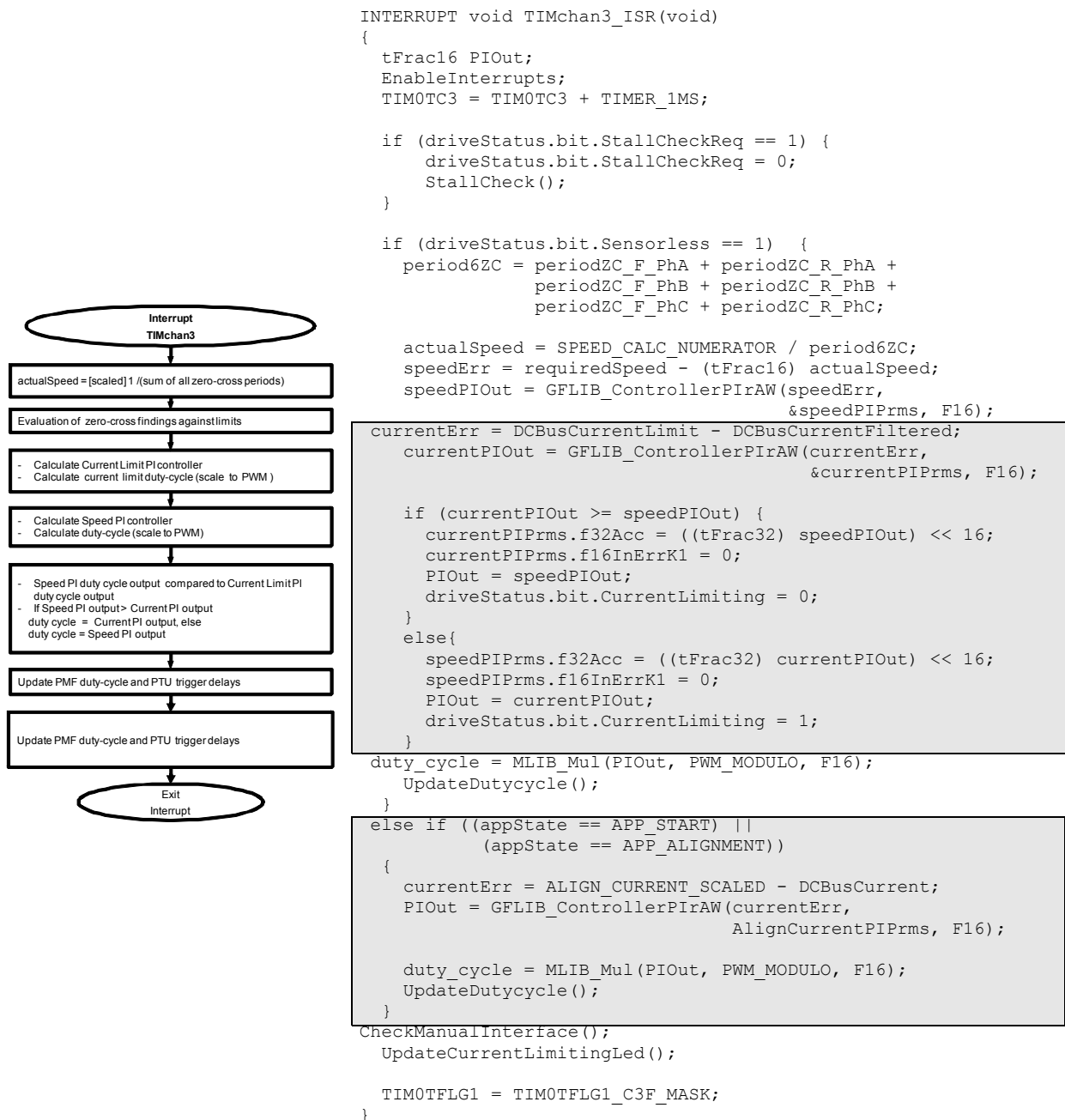
Figure 22. Speed evaluation and phase current limitation
