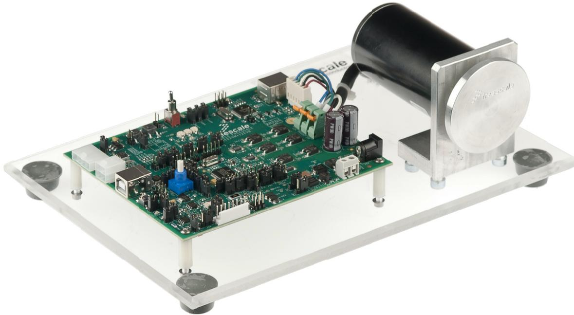
**Figure 2. 3-phase BLDC Motor Control Development Kit MTRCKTSBNZVM128**
