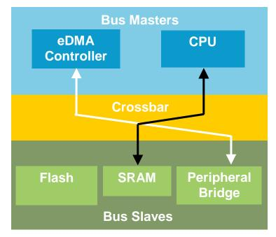
Figure 2. Multi-master bus architecture
