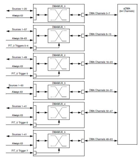
Figure 3. DMA channel multiplexing
